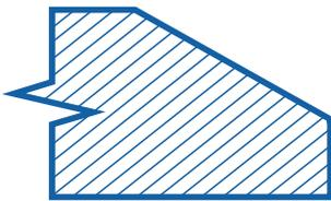
Bevel width 18 mm / 0.7 in - in first cut by feeding speed 1.8 m / min. / 5.9 ft/min.
